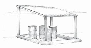
Simple storage sheds with a roof, liquid-tight floor and perimeter berm will usually prevent storm water from becoming contaminated.
