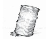
Tipping the drum minimizes liquid from collecting on top of drums.
