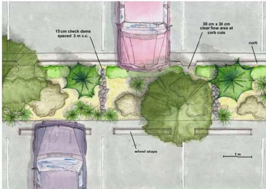
Figure 9 – An example of parking lot runoff draining to linear bioretention areas (Aqua-Tex Scientific Consulting Ltd.)
