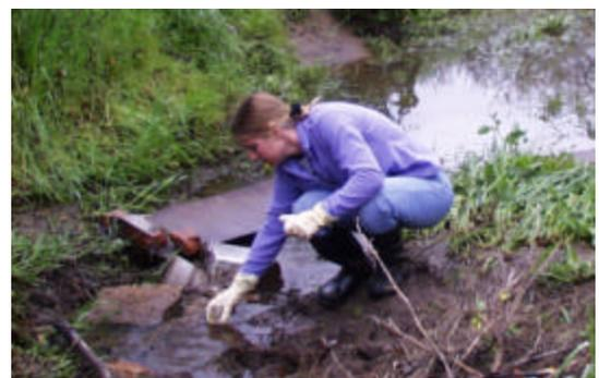
*Project Clean Water staff compiling samples of stormwater runoff*
